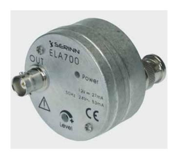
Small Video amplifier for Colour and B/W signal, made of Aluminium alloy, equipped with male BNC (video IN) and female BNC (video OUT). ELA700 can be mounted directly onto the camera BNC OUT and connected to the camera power supply through the supplied cable. ELA700 has a power ON Led indicator and linear output signal amplification trimming.
