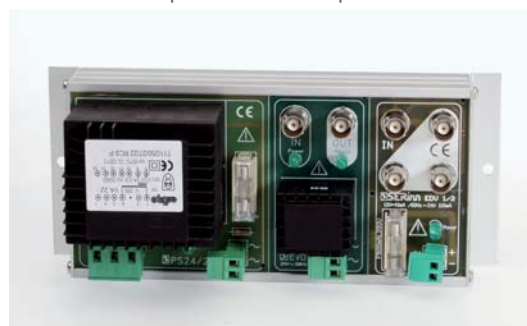
Detail of EV4/PS case complete with PS24/2M board, EVO1/1 board (opto) and EVD1/3 board (distributor)
