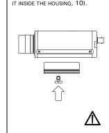
10) In order to fix the support: to press until embedding it from both sides.
